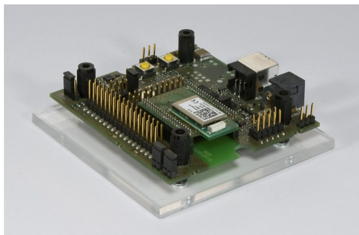
Figure 3: deRFnode-2TNP2 – board with radio module deRFmega128-22M00
