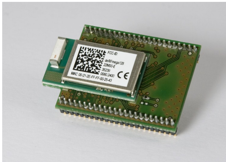
Figure 4: deRFmega128-22M00 mounted on an adapter board
